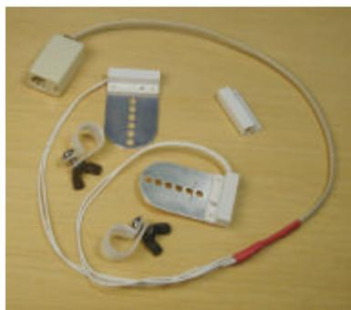
*Note: the switch unit was designed to operate on low-numbered TV channels, such as channel 3, normally used to carry the signal from the cassette player to the TV set. The switch will pass all normal analog cable*
